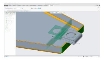
Recognize patterns of geometry in imported parts and propagate geometric changes to the pattern members
