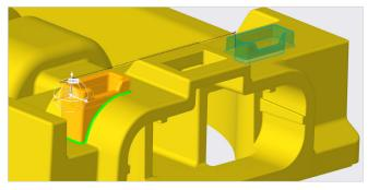
Flexible modeling helps you quickly edit geometry to your desired position by pushing and pulling the 3D Dragger
